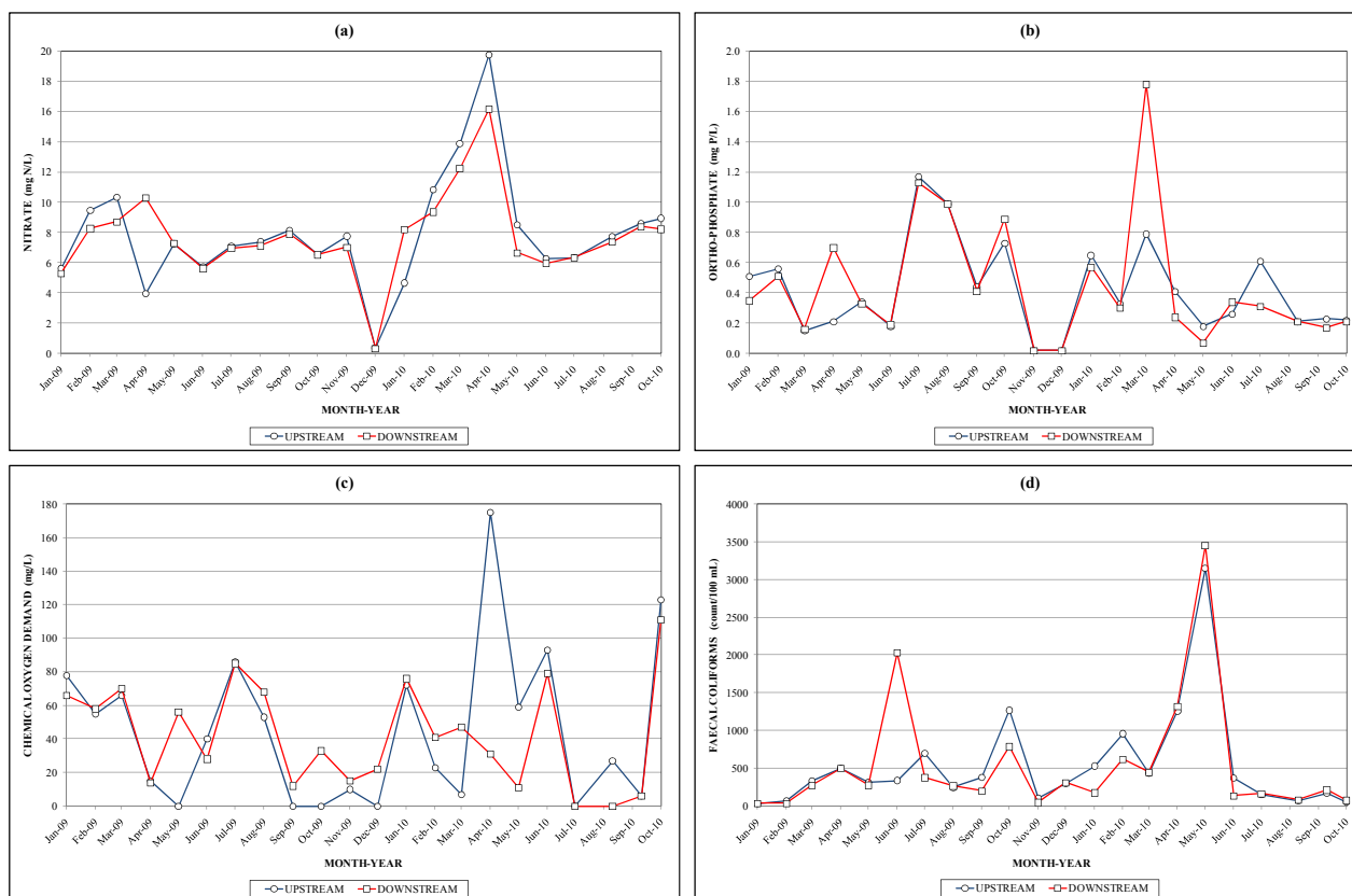
Figure 38. Recent temporal pattern of (a) NO 3 -N, (b) O-PO 4 -P, (c) COD and (d) faecal coliforms in Bloubank Spruit water at the Nedbank Olwazini Estate.
