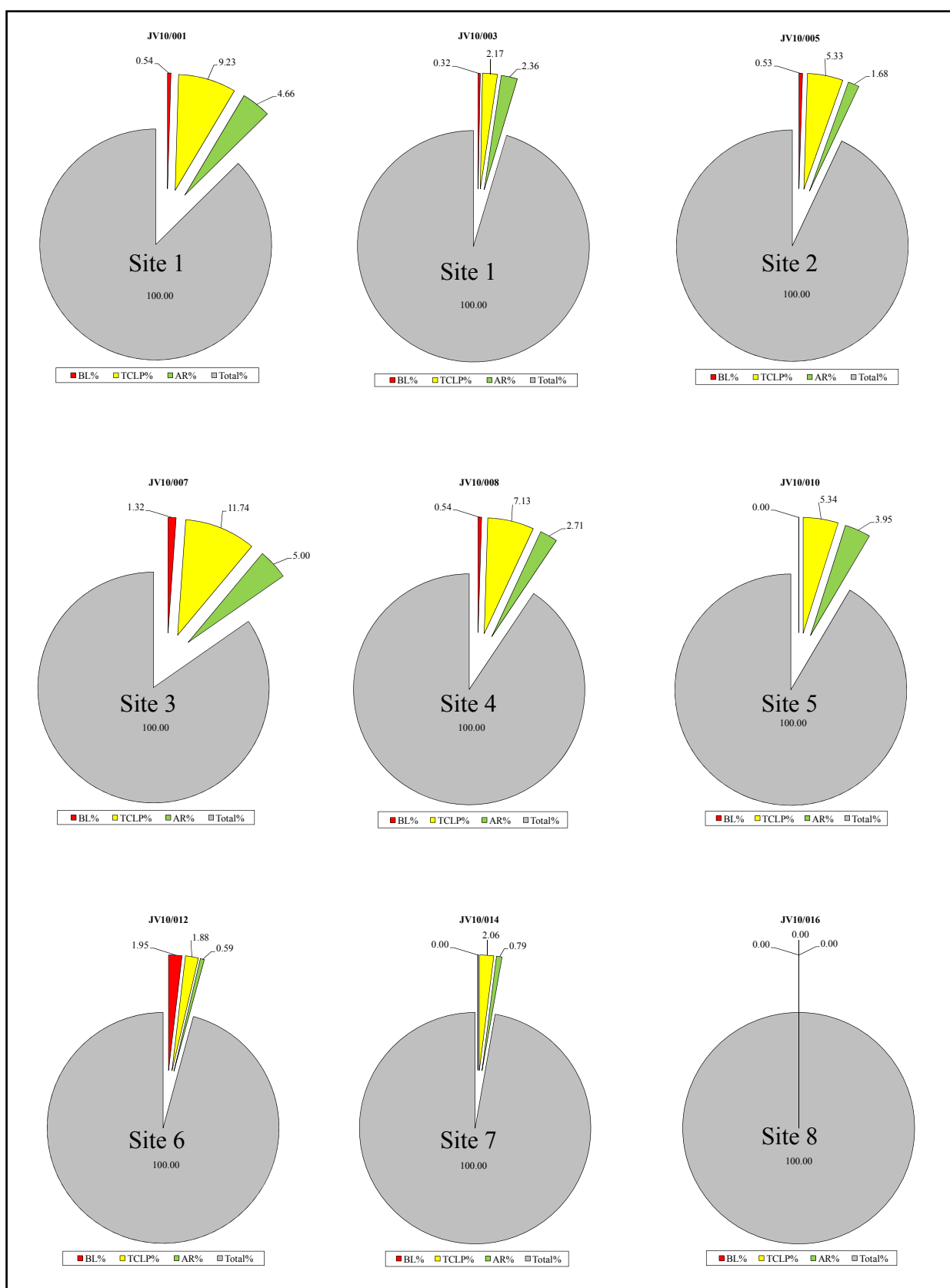
Figure 62. Pie charts of extractable (mobile) fractions expressed as a percentage of total nickel concentration per sediment sample as produced by the three leach test methods used. Note that each 'sliver' is a fraction of 100%.
