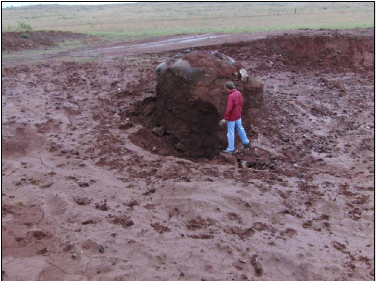
Unnumbered plate. Dolomite pinnacle protruding from a recently formed doline following flooding by stormwater of a soil borrow-pit for road construction alongside Dolomite Road. (Photo: Phil Hobbs)
