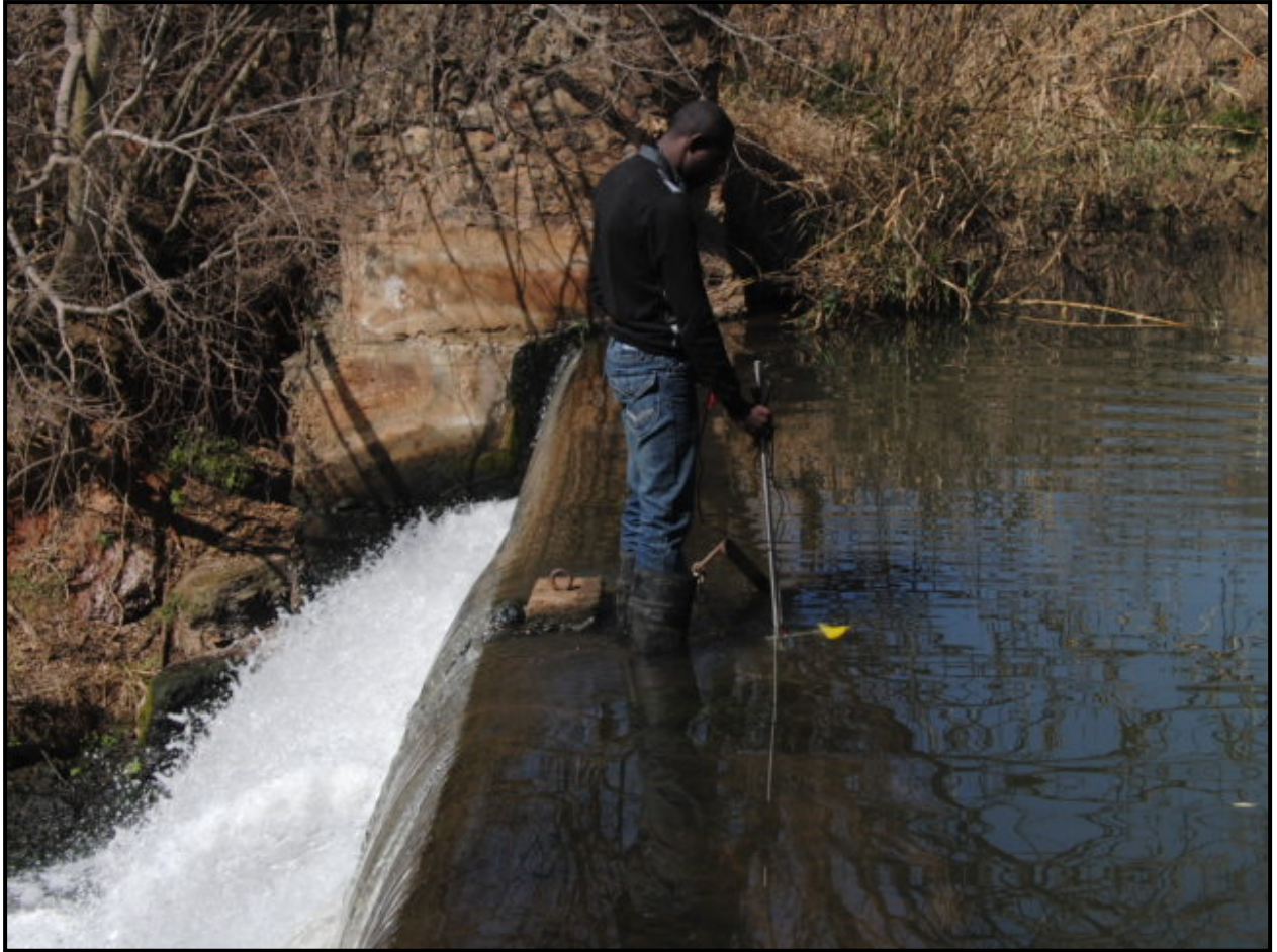
Unnumbered plate. Stream flow gauging at a weir on the Bloubank Spruit at Ekutheni Estate immediately downstream of the Kromdraai Spring. Flow on date of measurement (13/08/2010) ~547 L/s (~47.2 ML/d). (Photo: Phil Hobbs)
