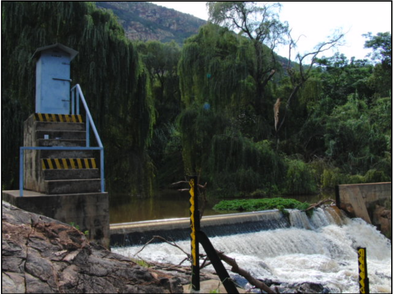
Unnumbered plate. View of DWA surface flow and water quality monitoring station A2H049 at the lower end of the Bloubank Spruit at Zwartkop showing hut housing automated stage gauging instrumentation at left, and vertical stage gauge plates in middle and right foreground for visual stage gauging observation. (Photo: Phil Hobbs)
